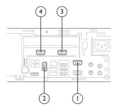
1 and 2: Powered Configurable serial port expansion card installation that supplies two additional serial ports (COM3 and COM4)
